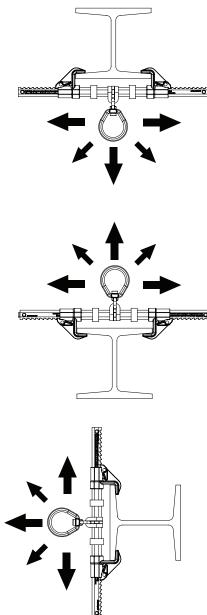
Placement at or below a user's working height requires integration of a compatible ANSI Z359.1 shock-absorbing lanyard that does not allow the user to extend more than 6 feet (in any direction) from the anchorage connector before the shock absorber is activated. The beam anchor must be attached to the l-beam flange facing the user (top flange if above, bottom flange if below, etc.).
